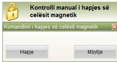
Fig 14. Manual command of the magnetic key from the computer
